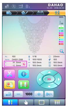
Press " key, to enter the interface for frame selection and position setting; then press " key, to enter the interface for setting related parameters, where user can input the coordinates of XY in the main interface.
